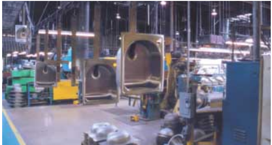
Formed and trimmed sinks ride the line at Elkay Manufacturing Co., Broadview, IL. At bottom sits stacks of untrimmed drawn sinks. For its trim dies, Elkay invested in powdered-metal tool steels for its cutting inserts. Compared to using D2 for the inserts, the number of hits between sharpenings has doubled.
