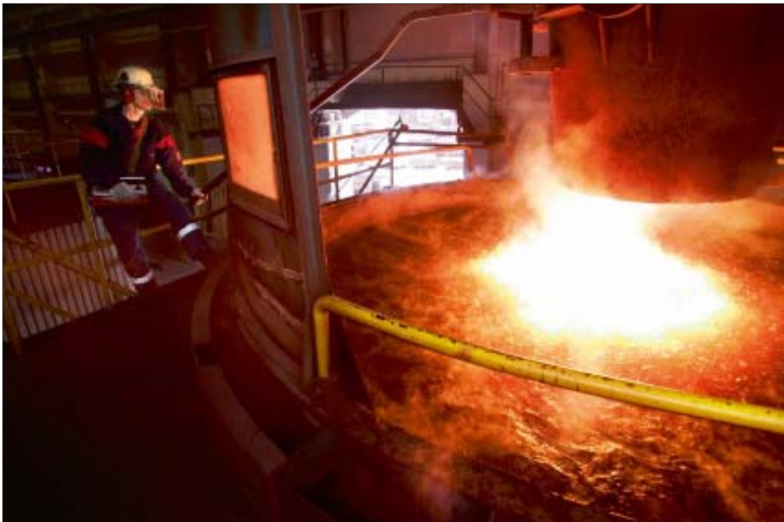
The Granshot granulation process.
